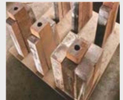
Magnesia Chrome Brick physical and chemical specification of Anode Converter (Copper smelting)
